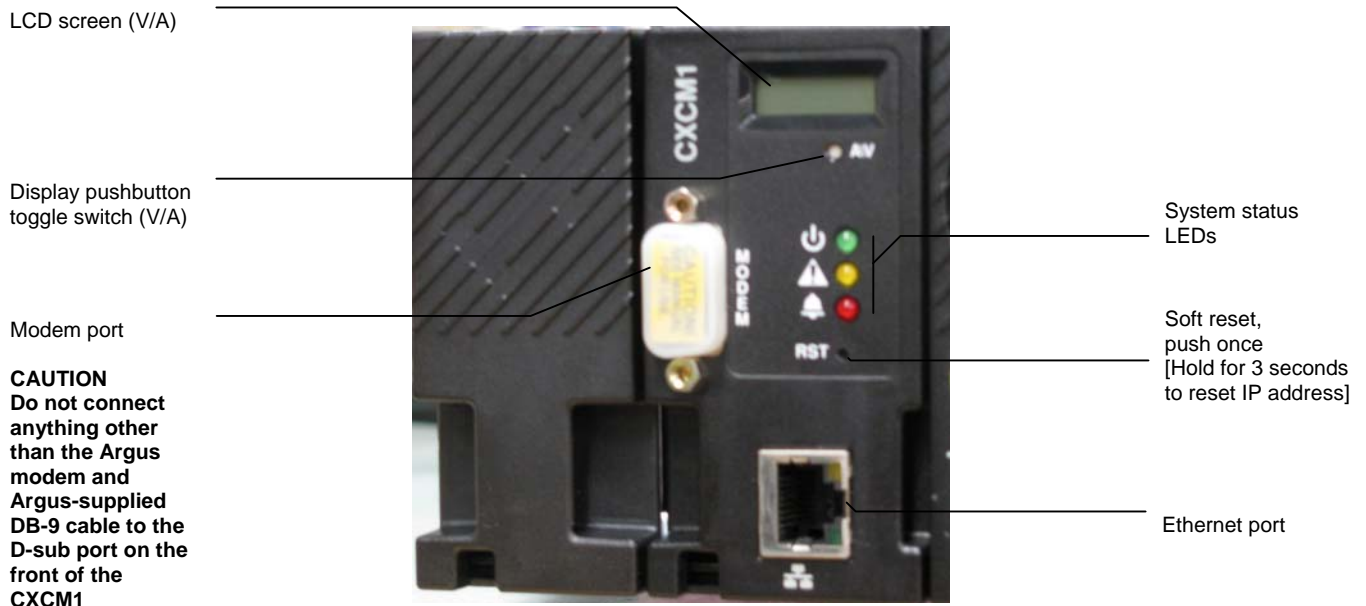
Figure 5–Cordex CXCM1 model system controller front panel
