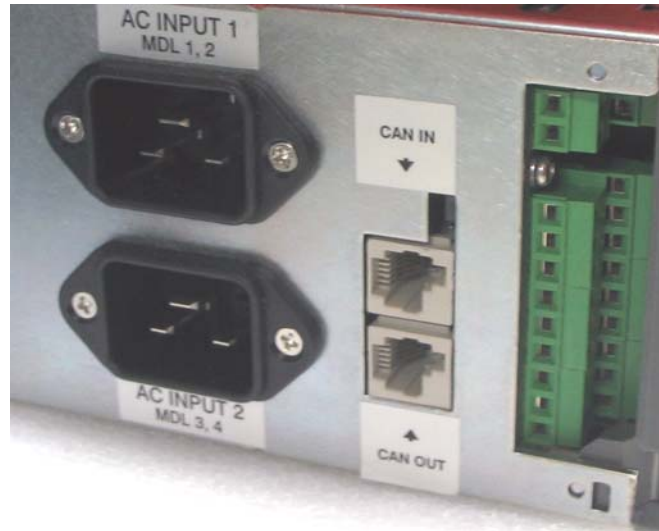
Figure 3–Cordex 48-1.2kW (4800W system) AC input, CAN, and signal connections
